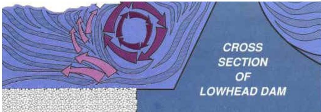
Cross Section of a Low Head Dam
